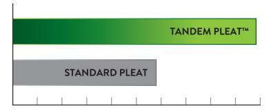
Tandem Pleat™ Construction provides 30% to 40% higher efficiency on particulate in the range of 0.3 to 0.7 microns. Dust loading tests confirm that Tandem Pleat™ filters can hold in excess of 40% more dust than conventional pleated filters.
