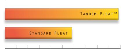
Tandem Pleat<sup>TM</sup> Construction provided 30% to 40% higher efficiency on sub micron particulate in the range of 0.3 to 0.7 microns. Dust loading tests confirmed Tandem Pleat<sup>TM</sup> filters to hold more than 40% more dust than conventional pleated filters.
